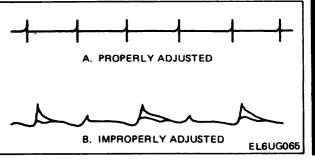
Figure 6-8. Inverter Balance.
