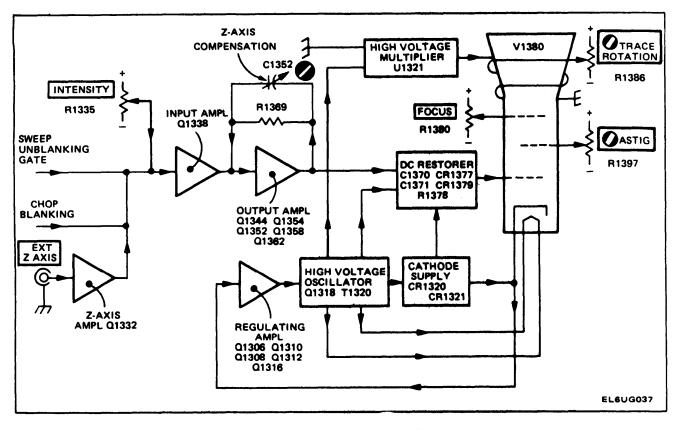
Fig. 3-10. Detailed block diagram of the CRT circuit.
