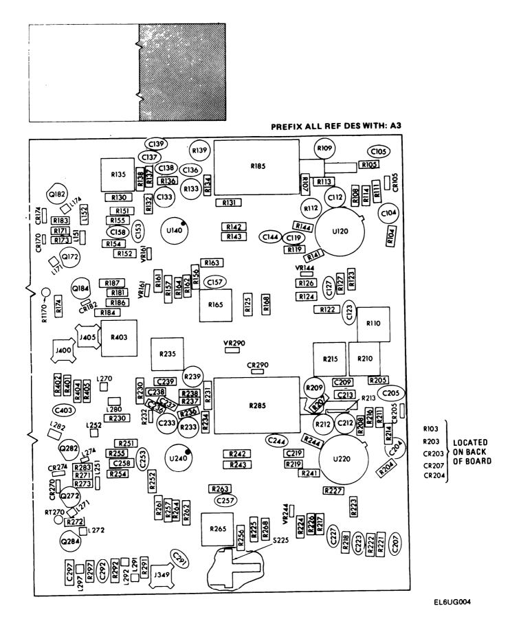
Fig. 7-2. A3 board component locations. (Sheet 2 of 2)
