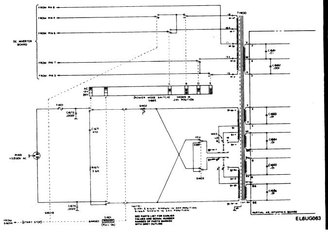
Figure 6-4. Option 07 primary winding.
