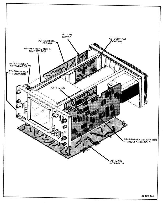
Fig. 4-5. Locations of circuit boards in the 475 Oscilloscope.
