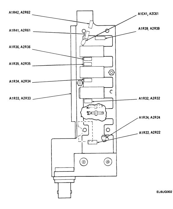
Fig. 7-1. A1 and A2 boards component locations.
