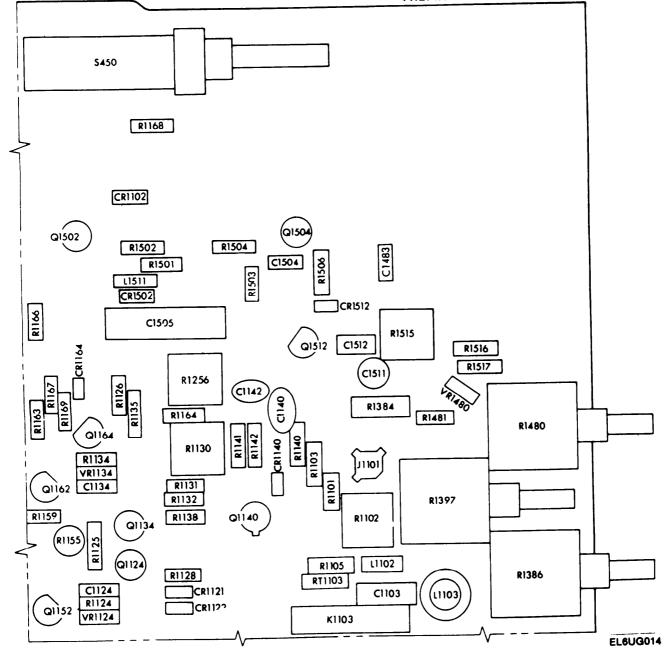
Fig. 7-8. A9 board component locations. (Sheet 3 of 6)
