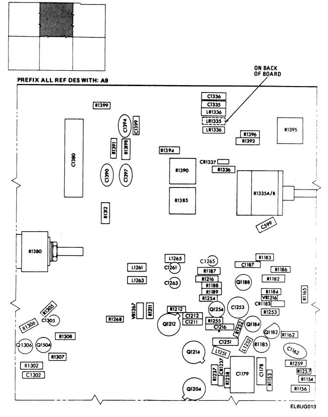
Fig. 7-8. A9 board component locations. (Sheet 2 of 6)
