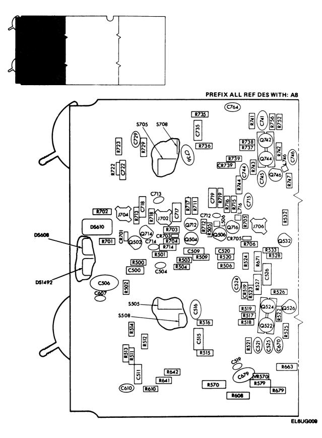
Fig. 7-7. A8 board component locations. (Sheet 1 of 3)
