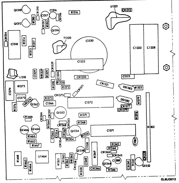
Fig. 7-8. A9 board component locations. (Sheet 1 of 8)
