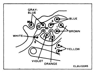
Fig. 4-6. Locations of power transformer secondary wires.
