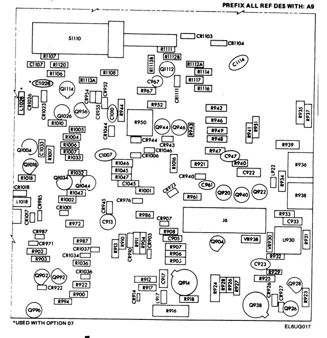
Fig. 7-8. A9 board component locations. (Sheet 6 of 6)
