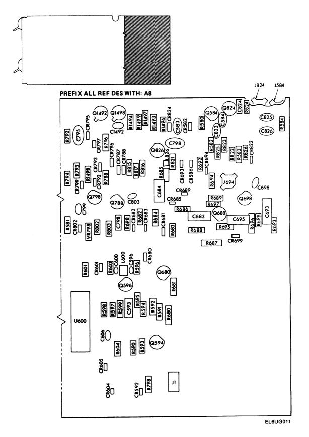
Fig. 7-7. A8 board component locations. (Sheet 3 of 3)
