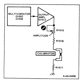
Fig. 3-11. Detailed block diagram of the Calibrator circuit.
