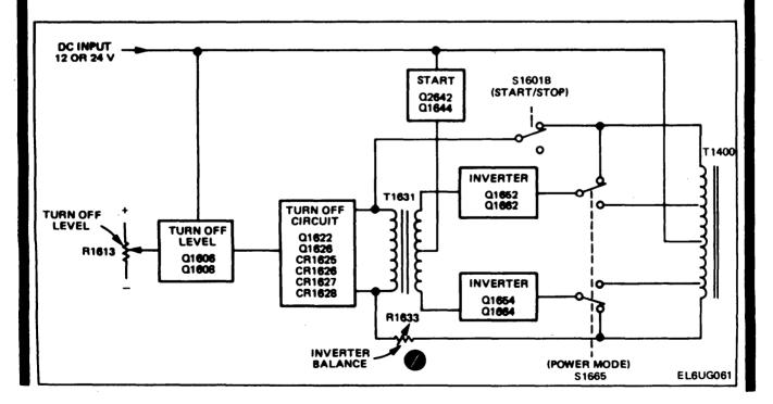
Figure 6-2. Option 07 simplified block diagram.
