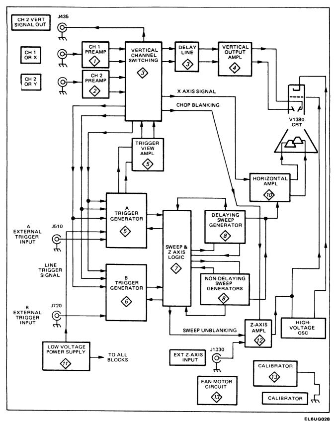
Fig. 3-1. Basic block diagram of the 475.
