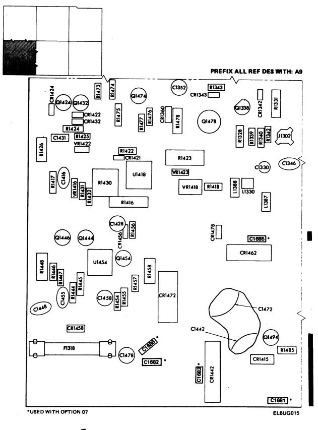
Fig. 7-8. A9 board component locations. (Sheet 4 of 6)
