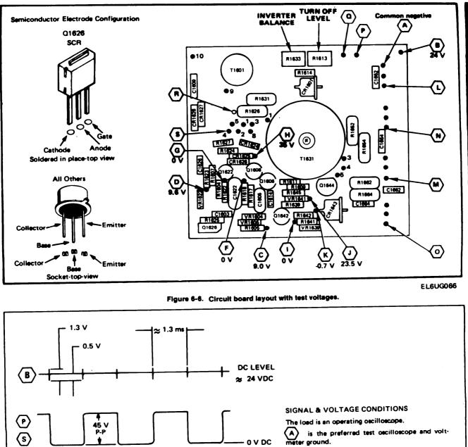
The voltmeter is a 20,000  $\Omega/V$  multimeter.
